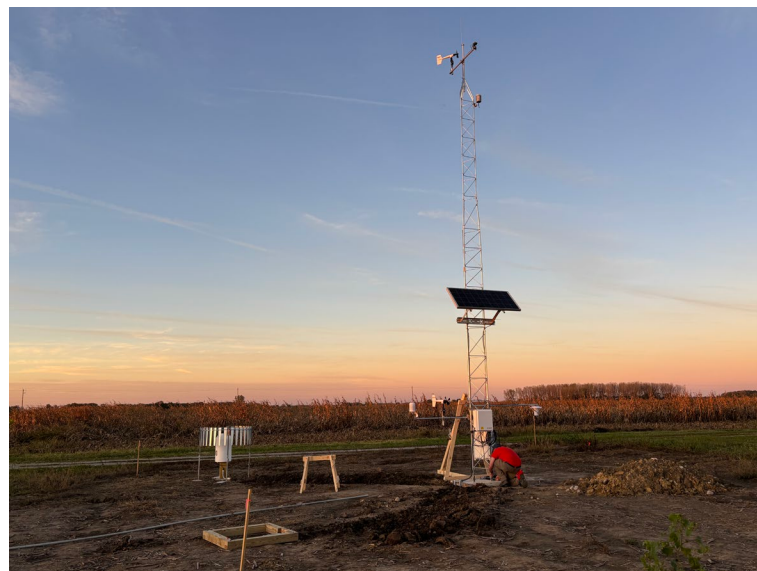
Figure 7: The South Charleston Mesonet station located at the OSU Western Agricultural Research Center. Courtesy of the Ohio State University Mesonet, a Network of Weather and Environmental Sensors, Supported by the State Climate Office of Ohio
