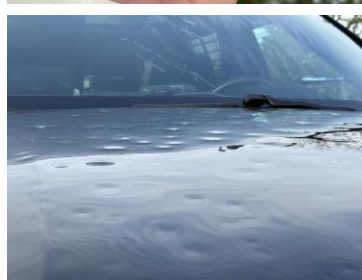
Figure 10. Solon police car damage from the April 15 hail storm. Solon police department. Accessed at https://www.news5cleveland.com/weather/weather-news/multiple-solon-police-cruisers-damaged-in-hail-storm
